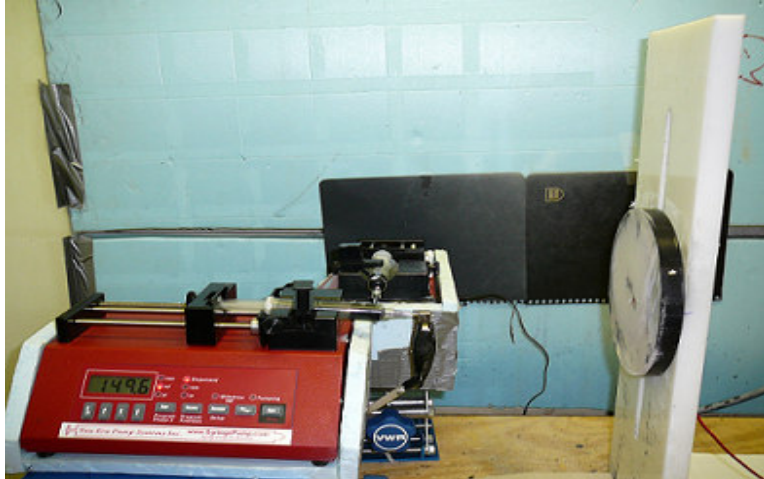
Figure 5. Electrospinning set-up for core-sheath nanofibers
