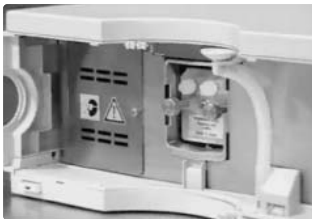
Front access to lamp and flow cell.
