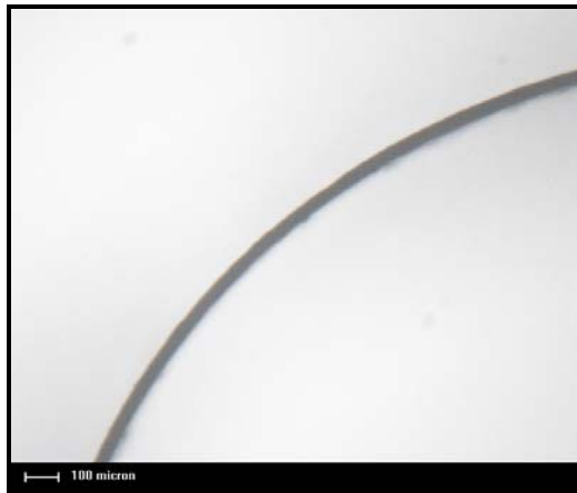
Figure 4.32-Cross-sectional image of an electrospun tube used for thickness measurement
