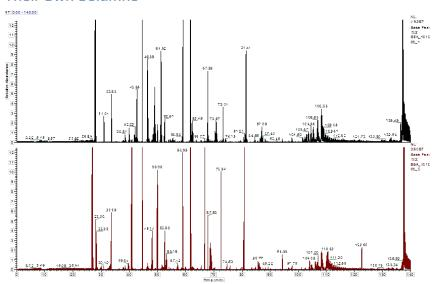
"We are very happy with the performance of our Next Advance pressure cell. Here are two representative total ion chromatograms generated from a capillary column using sub 2 micron, C18 particles and analyzed on a UPLC. As you can see the peak width is around 15 sec or less. We are getting this kind of resolution routinely from the columns packed by your pressure cell."
