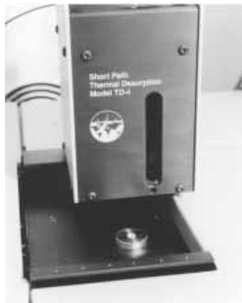
Fig 3.43 Align the S.P.T.D. unit over the septum nut adapter.
