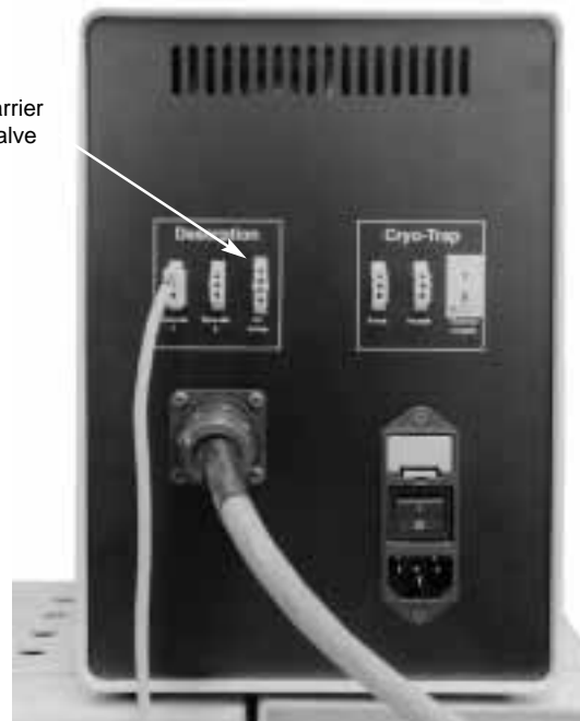
Fig 3.21 Plug the remote start cable into the plug labeled "Remote 1" on the rear of the S.P.T.D. controller.
