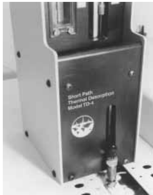
Fig 3.14 The S.P.T.D. fits snugly over the septum nut.
