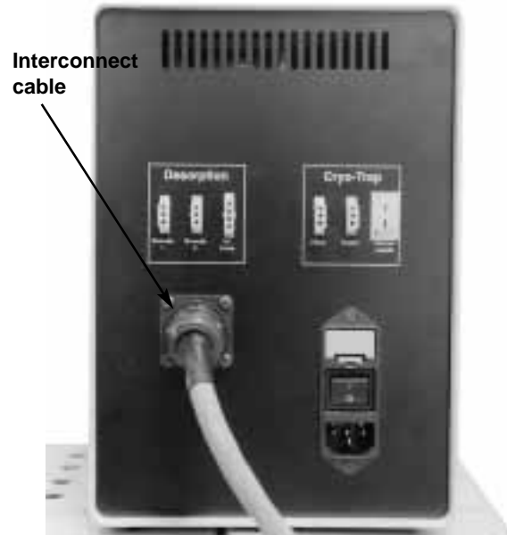
Fig 3.66 Installing the interconnect cable (782010).
