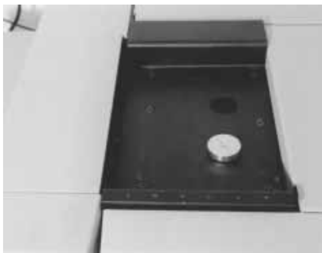
Fig 3.41 The septum nut adapter should sit firmly and evenly on the mounting plate.
