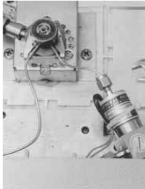
Fig 3.31 The solenoid valve must be installed in such a manner that it does not interfere with the GC injection port cover.
