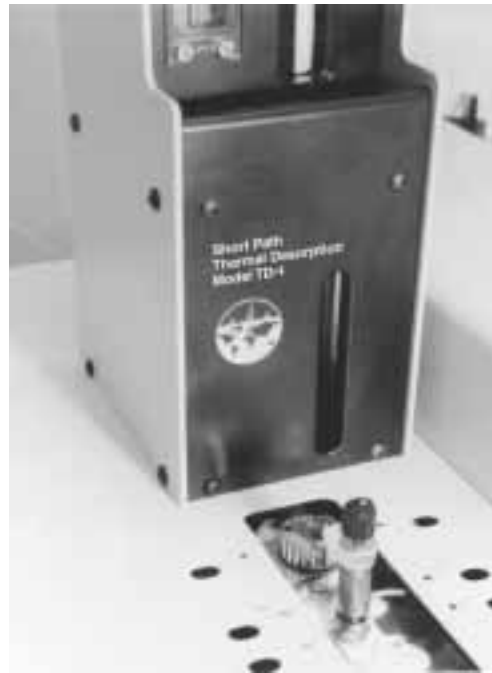
Fig 3.13 Align the S.P.T.D. unit over the septum nut.
